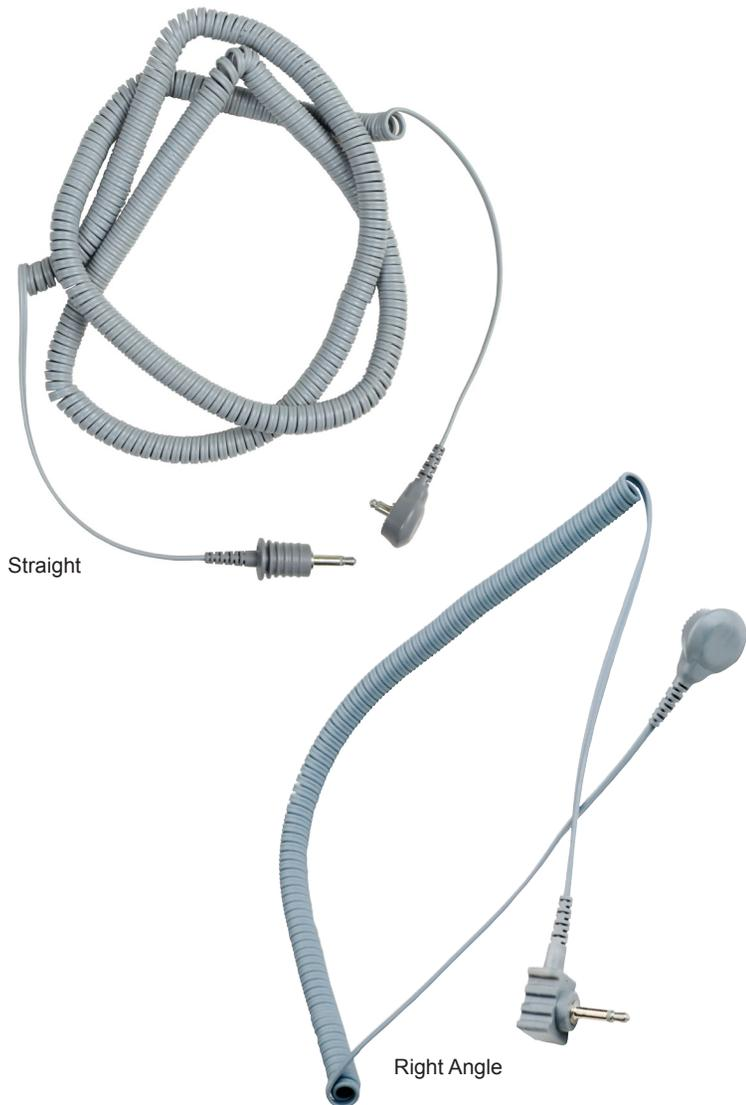
The 2300 Series Dual Conductor Coil Cord is for use with dual conductor wrist straps and SCS Workstation Monitors. The Dual Conductor Coil Cord features an improved grip that is wider in diameter and easier to grasp when inserting and removing the cord from the remote unit. Having a 1 megohm current limiting resistor (at the end to attach to the wrist band), the Coil Cord meets the resistance requirements of ANSI/ESD S20.20, EIA 625.
