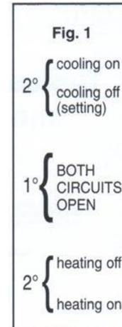
Model 22100 has a 1° F spread in which the heating and cooling switches are both open (see Fig 1). The two switches are so interlocked that they cannot both close at the same time. The thermostat can be used as either a heating or cooling unit by wiring one switch only.
