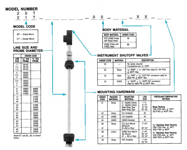
SERIES 20T—ACCUTUBE—SINGLE MOUNT. The Accutube Series 20T Standard Probe is constructed of stainless steel and brass. The Series 20T Probe has single-mounted support and installs through a single packing gland and thredolet. The Series 20T Accutube is factory-fitted with 1/8" FNPT connections and is shipped with mounting hardware complete. Series 20T Accutubes available for line sizes 1" through 30".
