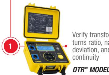
Verify transformer turns ratio, nameplate deviation, and winding continuity
