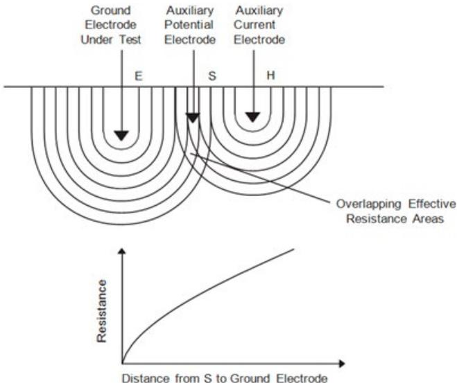
If readings were taken by moving the auxiliary potential electrode S towards either E or H, the reading differentials would be great and we could not obtain a reading within a reasonable band of tolerance. The sensitive areas overlap and act constantly to increase resistance as S is moved away from E.
