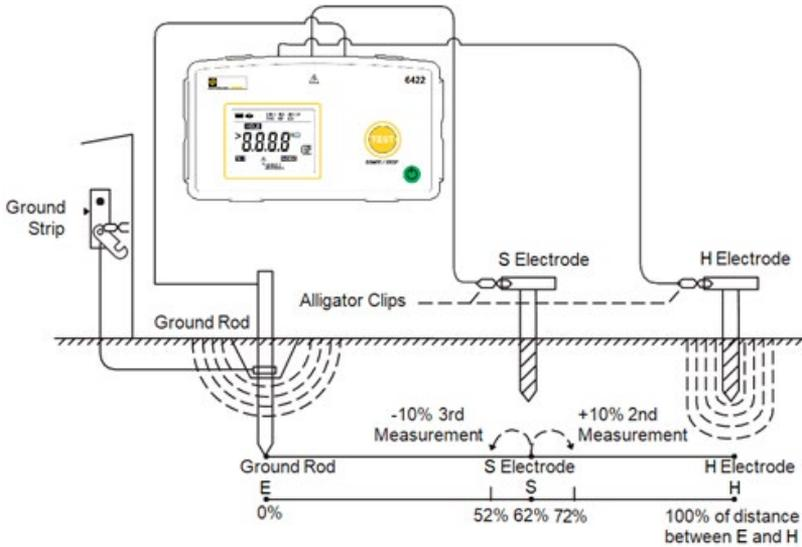
Consider the illustration below, which shows the effective resistance areas (concentric shells) of the ground electrode E and of the auxiliary current electrode H. The resistance areas overlap.
