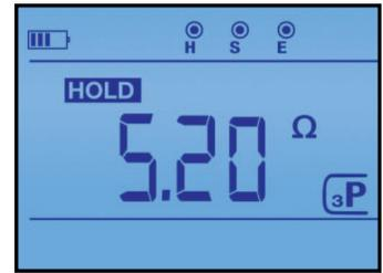
3 P mode used for measuring the grounding system. The resistance of the injector electrode and the test voltage are also displayed
