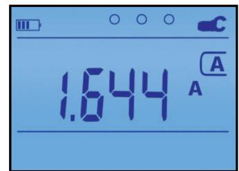
Leakage current is displayed when the optional MN72 probe is connected and the V/A function is selected (Model 6424)
