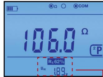
2 P mode used for continuity and bonding checks – is active when the instrument is turned on
