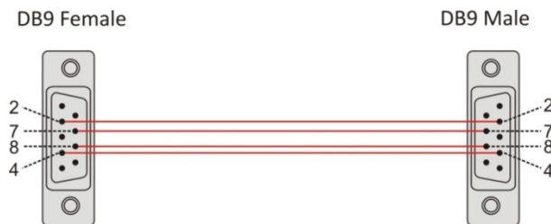
Figure 27 – Building an extension cable
