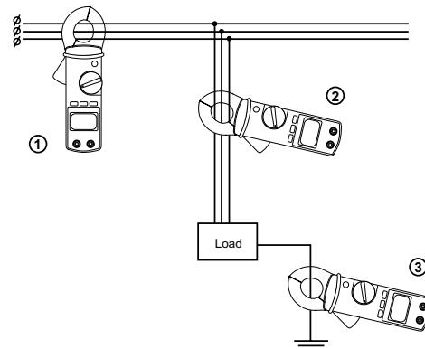
1. Measure branch leakage current (leakage from all loads on branch)
