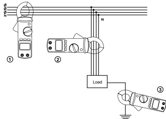
1. Measure branch leakage current (leakage from all loads on branch)
