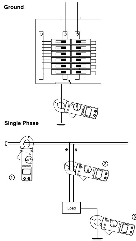
1. Measure branch leakage current (leakage from all loads on branch)
