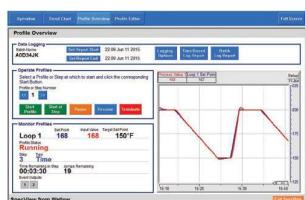
SpecView is designed for industrial users with features such as data logging, trending and support for bar code readers and touch screens. Errors are reduced, for any process, by creating application-specific screens. The software provides a
