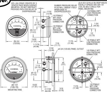
\*The blowout plug is not used on models above 180 inches of water pressure, medium or high pressure models,
