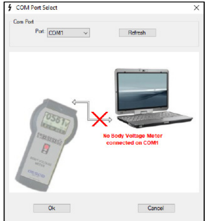
Figure 6. Selecting a COM port using the WT Manager software
