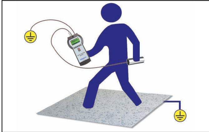
Figure 3. Setup of the Body Voltage Meter
