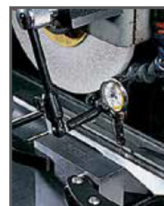
657A with 711LS Last Word Dial Test Indicator setting up workpiece on surface grinder.
