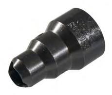
From Klein Tools, the Conduit Reamer works with a screwdriver to ream and smooth thin-wall conduit. It locks onto a screwdriver and can ream both ID and OD at the same time. Comes with two set-screws to fit either round or square-shank screwdrivers.
