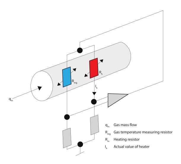
Tek-Thermal 1700B Thermal Mass Flowmeter design is based on constant power measuring method, thus the RTD is heated on a consistent power and will be more durable and stable. Due to that, Tek-Thermal 1700B has less problem of zero-off which may cause a function failure of RTD due to overheating the term.
