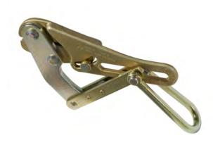
Designed for use on aluminum, copper, weatherproof coated wire, PVC covered conductors and messenger and guy strand. The Chicago style grip was designed for cable sizes from 0.218-Inch to 0.55-Inch (5.54 to 13.97 mm). When pulling EHS (extra-high-strength) galvanized-steel cable, the galvanizing has a tendency to coat the jaws of any grip, causing the cable to slip. Double "V" contour reduces the possibility of slippage and damage to the cable
