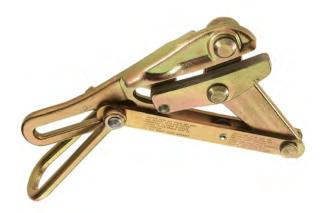
Designed for use on aluminum, copper, weatherproof coated wire, PVC covered conductors and messenger and guy strand. The Chicago style grip was designed for cable sizes from 0.12-Inch to 1.0-Inch (3.10 to 25.4 mm). When pulling EHS (extra-high-strength) galvanized-steel cable, the galvanizing has a tendency to coat the jaws of any grip, causing the cable to slip. Double "V" contour reduces the possibility of slippage and damage to the cable.
