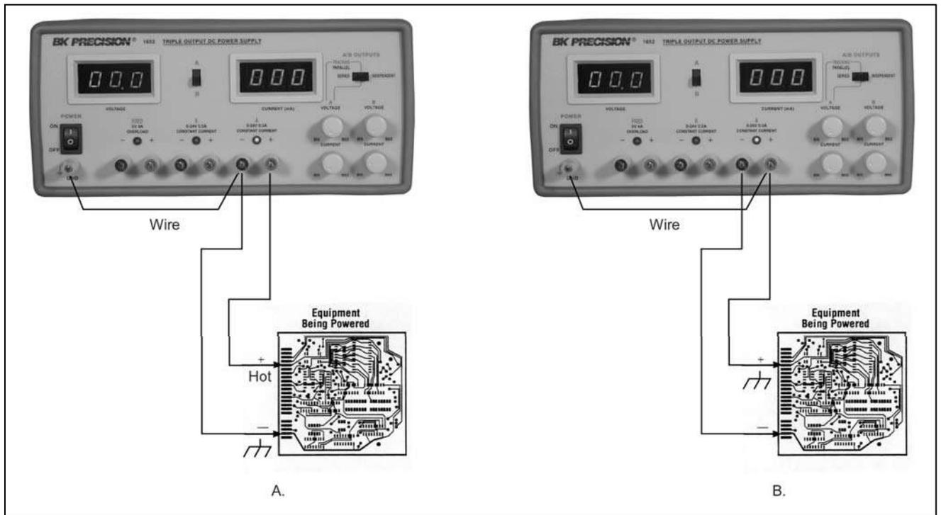
**Figure 3. Independent operation grounding possibilities (sheet 1 of 2)**
