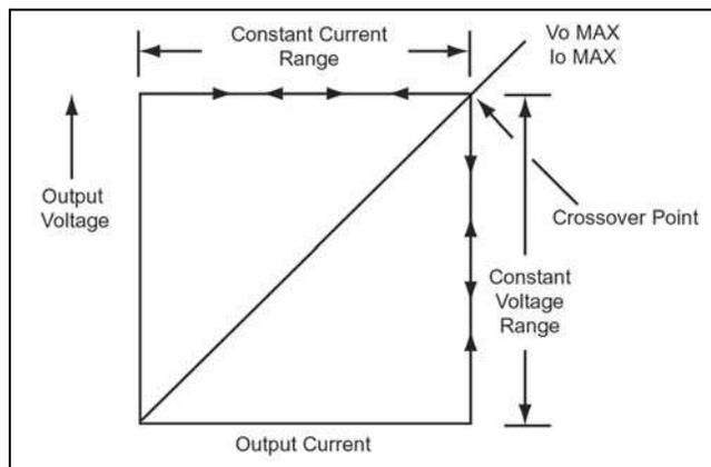
Figure 7. Constant voltage/constant current characteristic.
