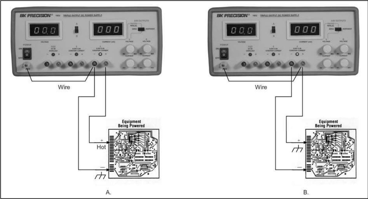
Figure 9. Parallel tracking operation grounding possibilities (sheet 1 of 2).
