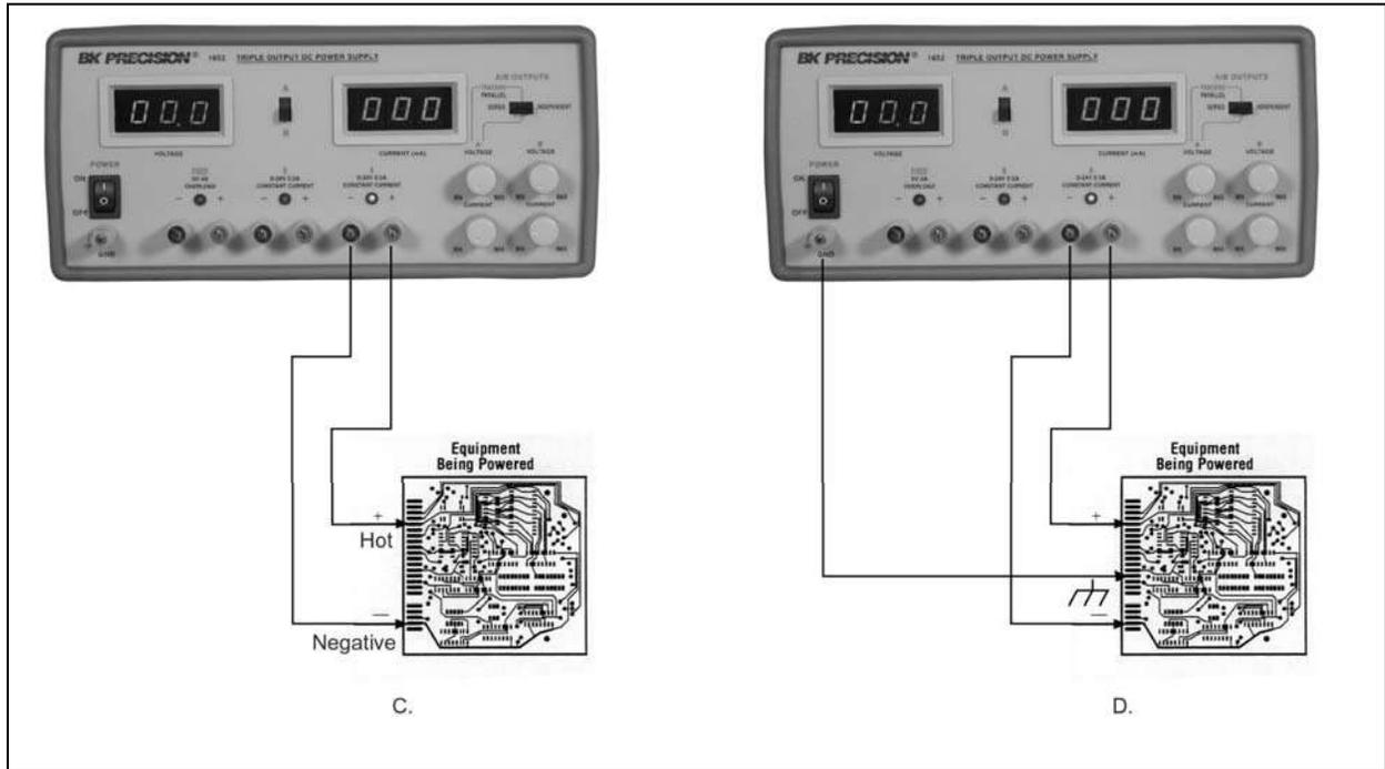
**Figure 9. Parallel tracking operation grounding possibilities (sheet 2 of 2).**
