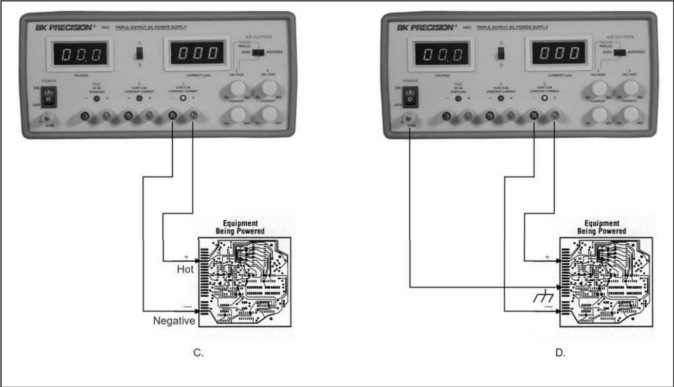
Figure 3. Independent operation grounding possibilities (sheet 2 of 2)
