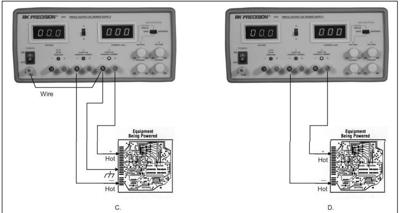
Figure 8. Series tracking (0-48 V) operation grounding possibilities (sheet 2 of 3)
