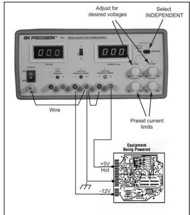
**Fig. 16. Typical Hook-Up Using Different Positive and Negative Voltages and a Separate Common.**
