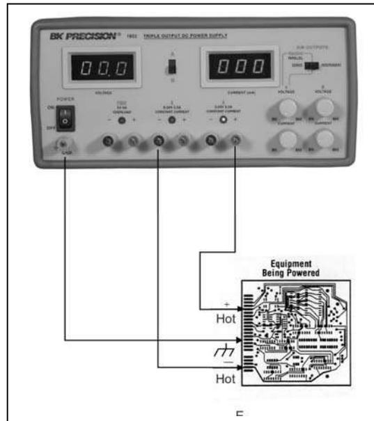
**Figure 8. Series tracking (0-to-48 V) operation grounding possibilities (sheet 3 of 3).**
