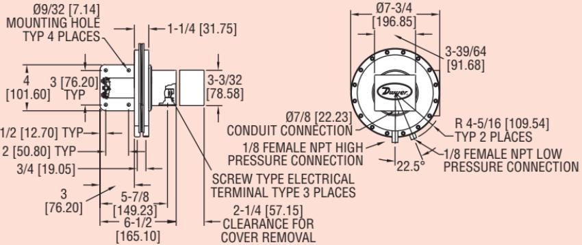
**The unique electric switch design in the 1640 is another Dwyer Instruments, Inc. innovation.** The Dwyer® Model 1640 Differential Pressure Switch resembles the Series 1630 switches. However, the 1640 is equipped with a single pole, double throw floating contact switch (not snap acting) so it functions as a null switch.
