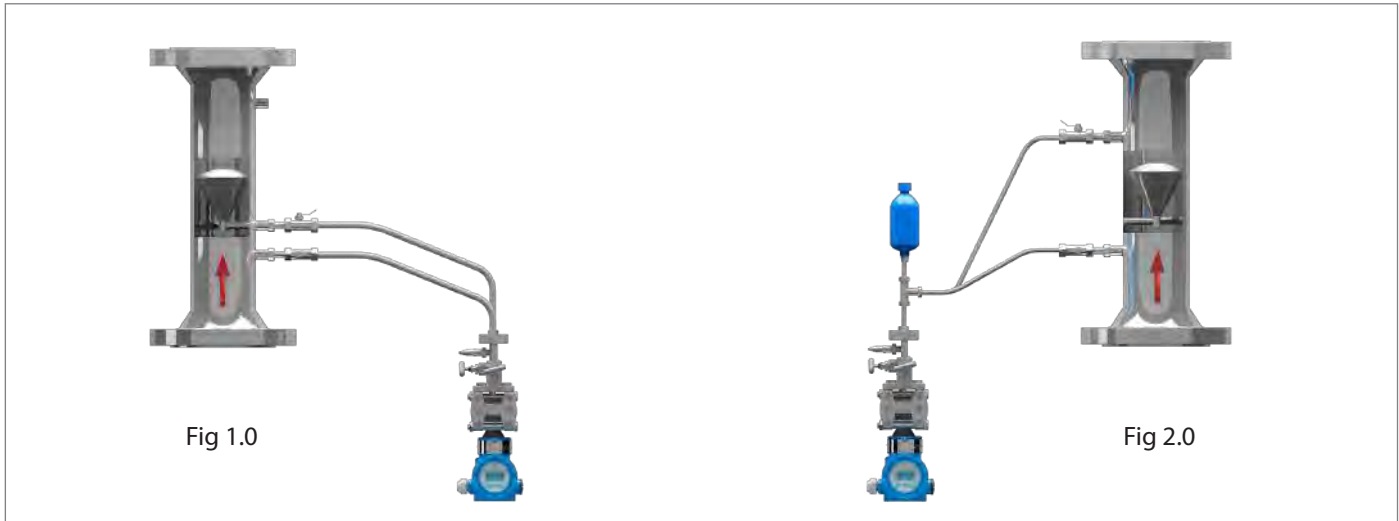
Fig 6: Installation suggestion for upward flowing condition - Cone Meter with Vertical Orientation
