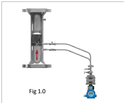
Fig 8: Installation suggestion for upward flowing condition - Cone Meter with Vertical Orientation
