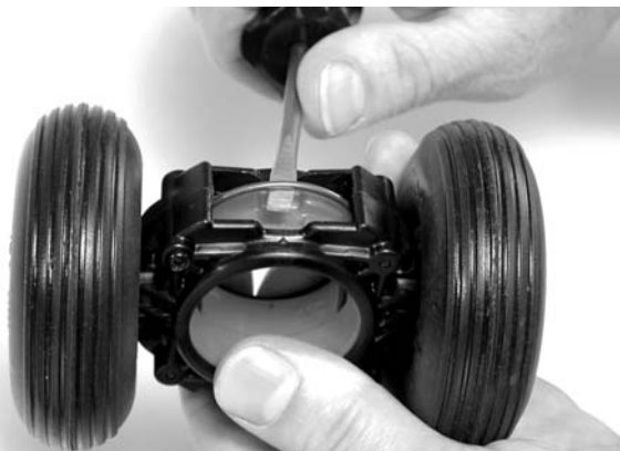
Figure 20 – Opening The Roller Dolly Retaining Rings
