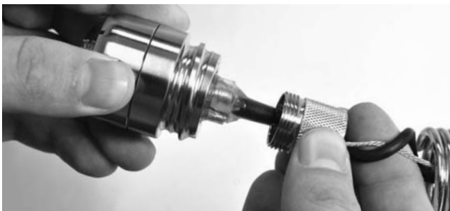
Figure 37 – Separating Locking Sleeve From Camera Head
