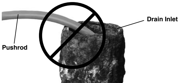
Figure 33 – Avoid Pulling At Sharp Angles
