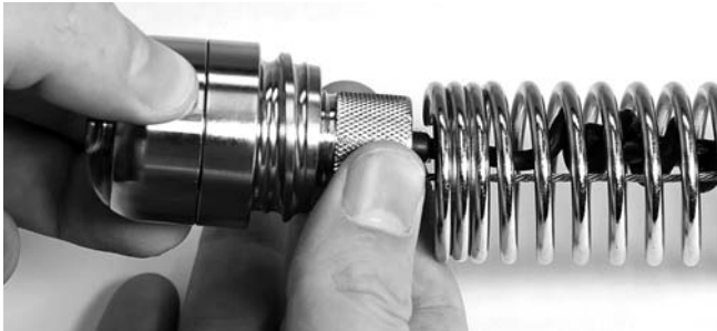
Figure 36 – Removing Camera Head From Locking Sleeve
