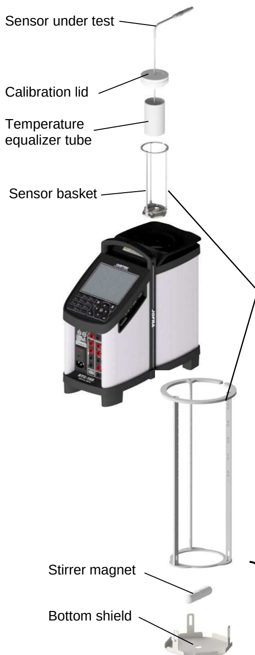
Fig. 2a Inserting the liquid bath kit RTC-168
