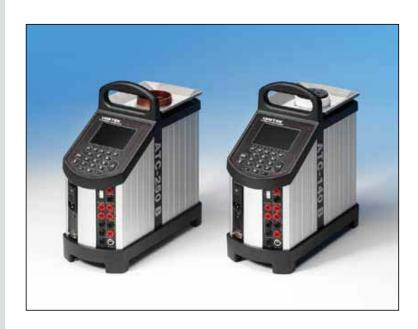
The JOFRA ATC series (Advanced Temperature Calibrators) combines the accuracy of laboratory temperature sources with the speed and portability of field dry-block calibrators.
