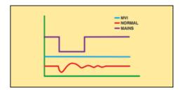
The JOFRA ATC-250 calibrator employ the MVI, thus avoiding such stability problems. The MVI circuitry continuously monitors the supply voltage and ensures a constant energy flow to the heating elements.
