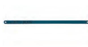
The Klein 1232BI-P bi-metal blade has special high-speed steel teeth that are fused to regular a carbon-steel body to provide superior cutting and a longer life. It withstands greater saw tension for less blade flexing. It fits all 12-inch hacksaw blades.
