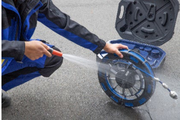
Fig. 57: Cleaning the viper and the rod
