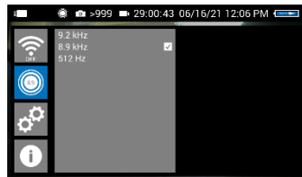
Fig. 32: Locator detection with 8.9 kHz transmission frequency selected
