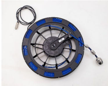
Fig. 56: Viper removed from the case, monitor plug covered by a lid
