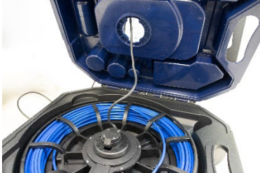
Fig. 60: Wrong: Camera cable not pulled tight
