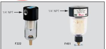
Compressed air filters protect equipment and instrumentation from harmful contaminant's such as dirt, water and oil. Liquids are continuously coalesced and released through the manual drain valves. Replaceable filter element removes particles and droplets as small as 0.01 micron with 93% efficiency. Units have 1/4′ female NPT inlet and outlet and manual drain valve.
