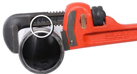
Figure 4 – Wrench Too Small For Work Piece, Hook Shank Touching Work Piece.
