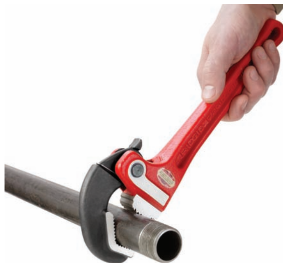
Figure 5 – Using a RapidGrip Wrench
