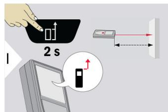
Distance is measured from the front of the device.
