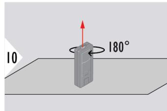
Turn the device horizontally by 180° and place it again on absolutely flat surface.
