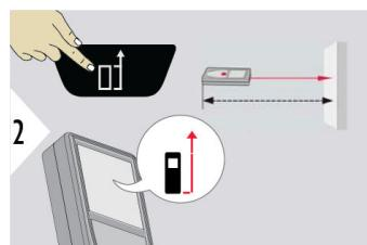
Distance is measured from the rear of the device (standard setting).
