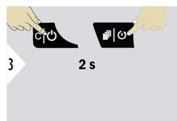
Press both keys simultaneously. Memory is completely deleted.
