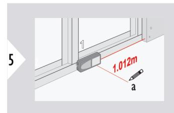
Start measuring. Move device slowly along the stake out line. The distance to the previous/next stake out point is displayed.
