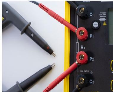
*\*For Models 6240 and 6255 instruments with serial numbers lower than 1166339SEDV, terminals C1 and P1 are red, and C2 and P2 are black. In this case, connect probes as shown in the table on the following page.*
