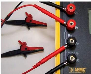
For the probes with **Red/Blk** and **Red/Blk** leads and **Red DOT** located on the probe tip: Connect them as shown here.
