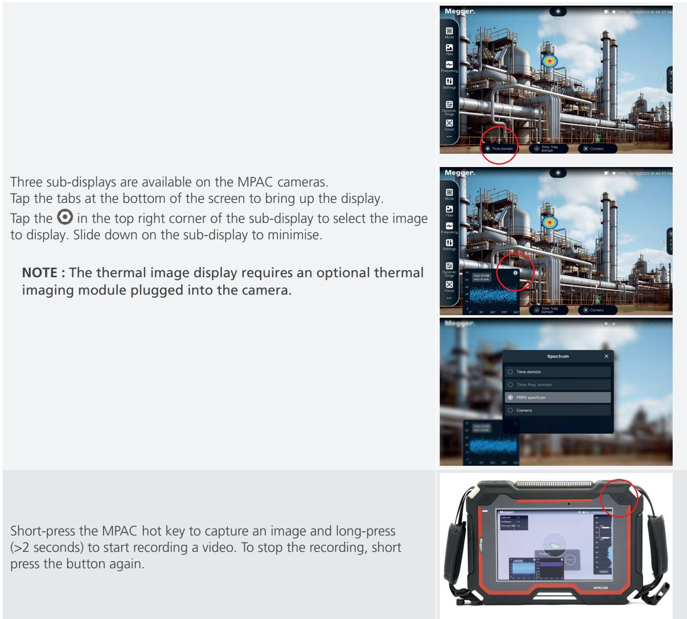
Three sub-displays are available on the MPAC cameras. Tap the tabs at the bottom of the screen to bring up the display. Tap the
