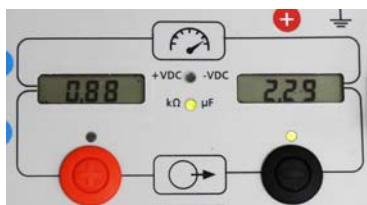
Some of these circuits would be expected to read OL, with very high impedances. When a fault occurs, use the transmitter to read the impedance of each circuit and compare them to the un-faulted impedance. This can help you locate the circuit that has changed and has the fault.
