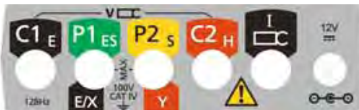
Test lead connections (at rear of instrument)
