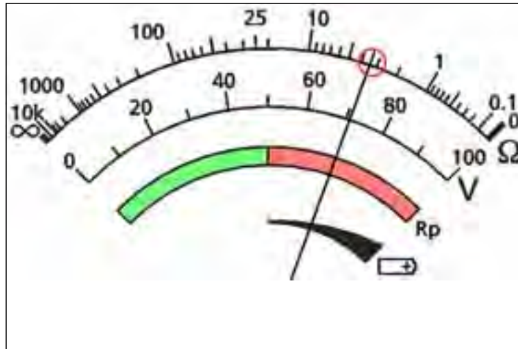
Figure 17: example two-terminal resistance reading
