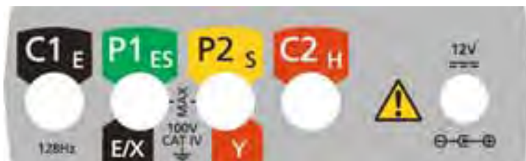
Test lead connections (at rear of instrument)
