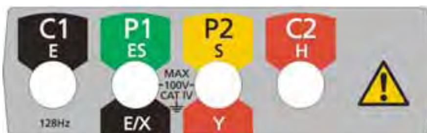
Test lead connections (at rear of instrument)
