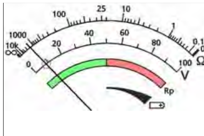
Figure 21: ground noise voltage indication
