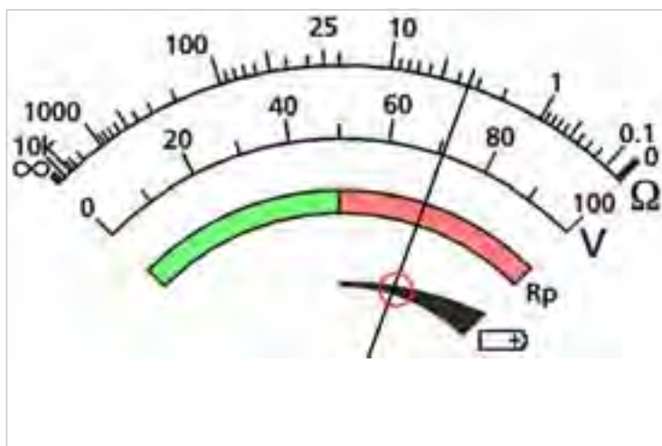
Figure 1: battery charge level indicator
