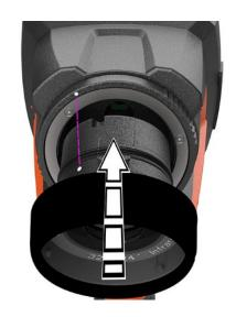
Align the markings on the lens and handle.
