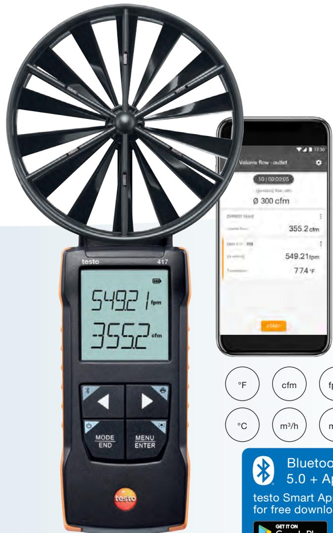
The compact testo 417 4 inch vane anemometer was developed to ensure precise results when measuring air inlets and outlets of **air conditioning and ventilation systems**. Time and point average values as well as the volume flow are automatically calculated in the instrument and shown on the display.
