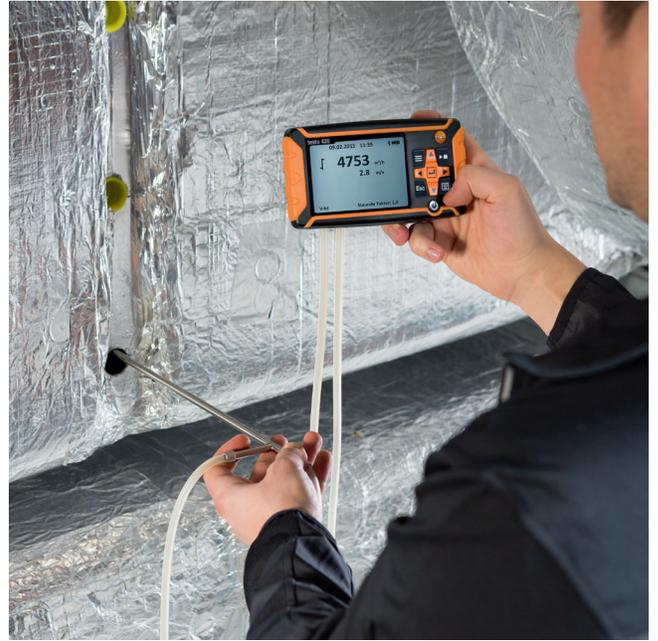
Removable instrument allows Pitot tube measurements in ducts (Pitot tube optional)
