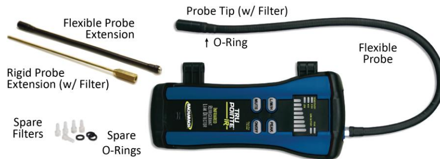
Figure 6. Flexible and Rigid Probe Extensions
