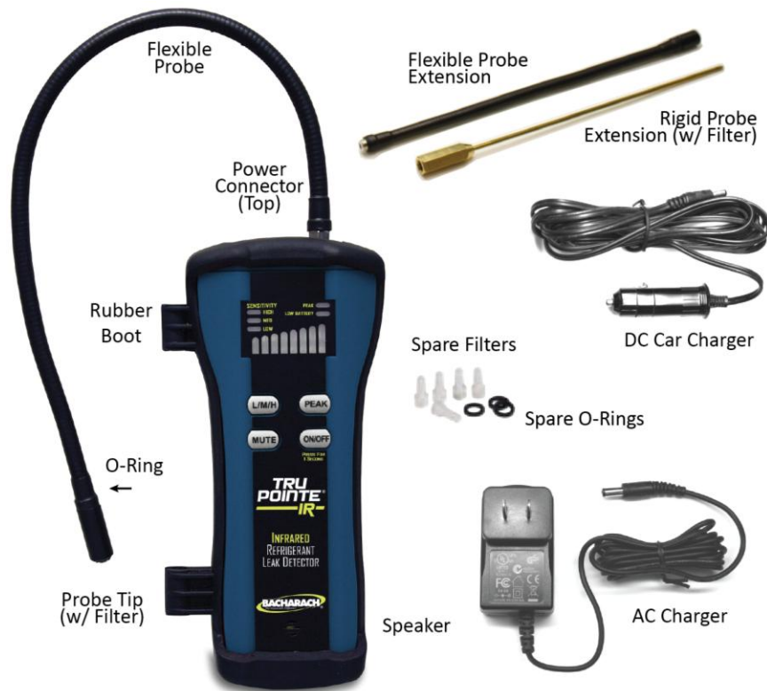
Figure 2. Tru Pointe® IR Components
