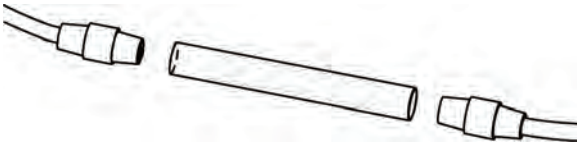
Figure 11. Removing End Plugs from Saturator Filter Tube
