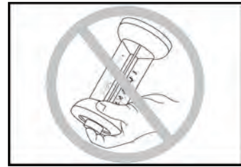
Figure 4. Never Vent FYRITE® in the Inverted Position (Causing Fluid Spillage)
