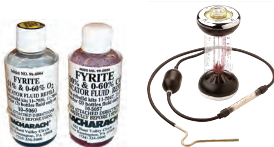
Figure 7. Chromous Chloride (Blue) and Potassium Hydroxide (Red) Reagent Fluids
