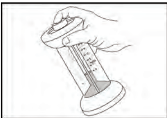
Figure 3. Venting FYRITE® to Atmosphere at 45° Angle
