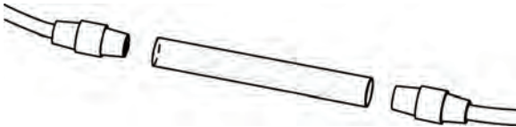
Figure 11. Removing End Plugs from Saturator Filter Tube
