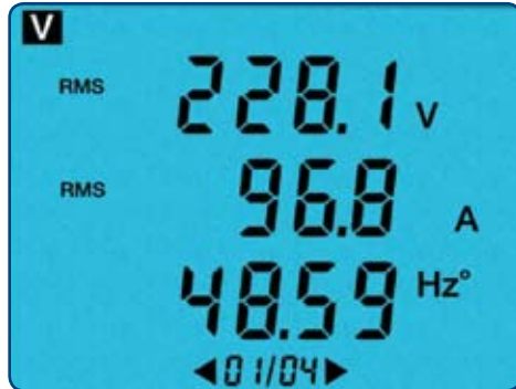
Displays volts, amps and frequency on one screen.
