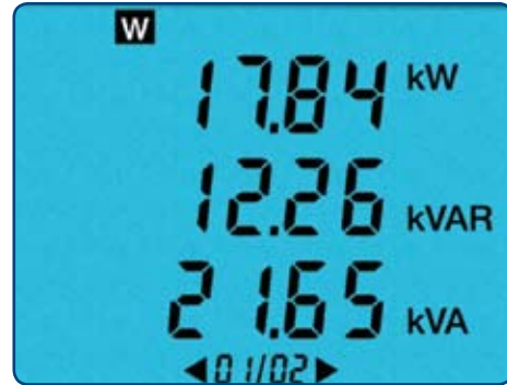
Displays all power measurements on one screen.
