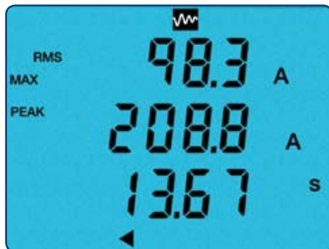
Displays inrush current and duration including max and peak values.
