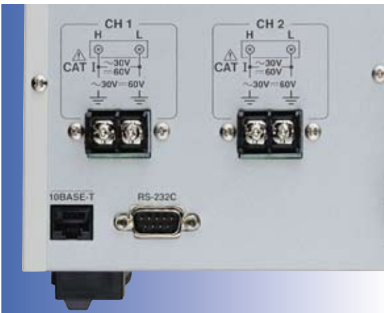
Rear view (input terminals)
