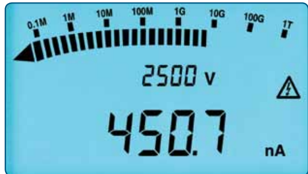
Leakage Current Measurement from 1pA to 3000μA displayed during the test .
