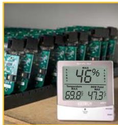
Indicates Humidity and Temperature levels in Production areas.
